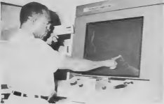
To have a view of the complete drawing, W. Wilson will insert one of those IBM aperture cards he is displaying in the aperture card machine in front of him.
